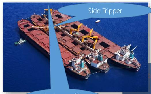
2 luffing and rotating shiploader 3000 t/ph each
