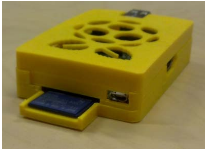
Figure 10: 3D Printed modified RPi case with memory card shield
