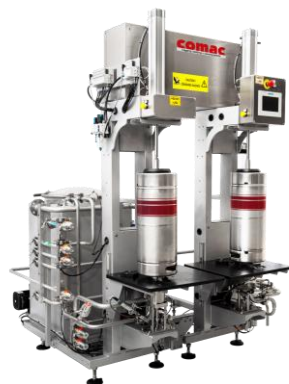
K2 SMART KEGGING MACHINE (30 KPH)
