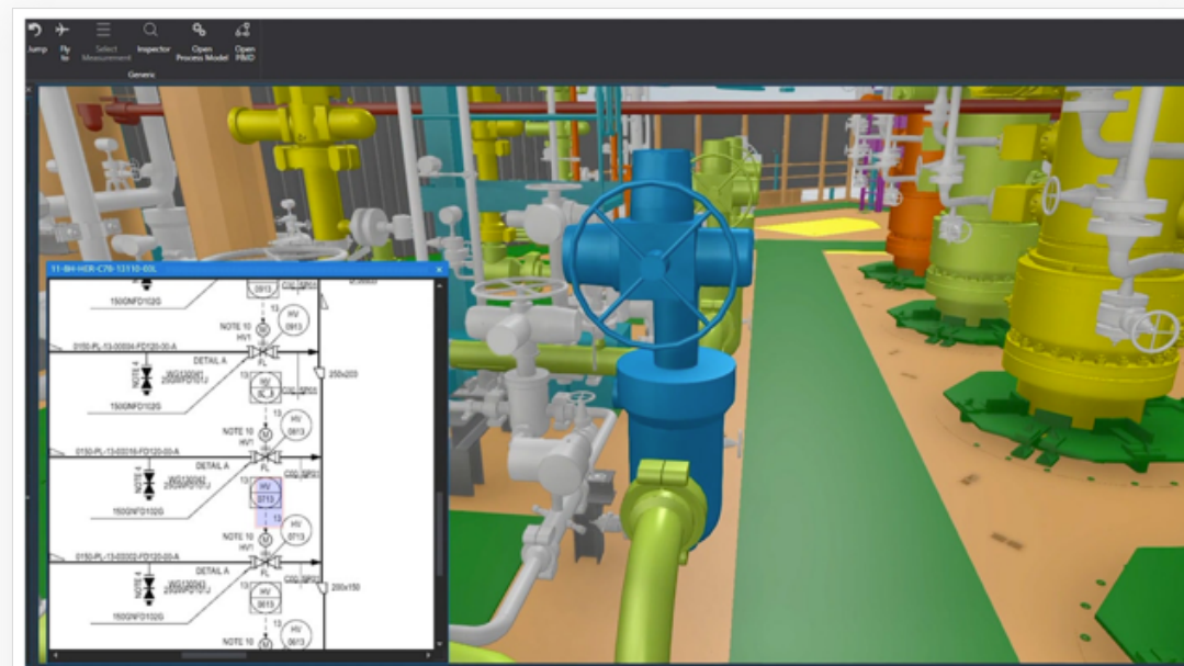
FIGURE 1. A working digital twin of an offshore oil platform. Screenshot from Kongsberg Digital's Dynamical Digital Twin for oil and gas, demonstrating interlinked 2D process diagrams and 3D visualizations of an oil and gas production facility enriched with real-time data from the asset. The color on the pipes shown in the 3D rendering can be used to show data such as flow rates, water / gas / oil fractions etc. The Dynamical Digital Twin can also run and explore what-if scenarios generated by process simulators in which case it will be more appropriately called a Digital Sibling. Copyright Kongsberg Digital 2019.
