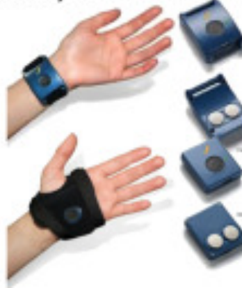
Electrodermal Activity (EDA) with Q-Sensor
